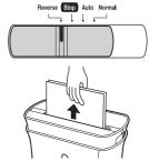
· If the paper cannot be removed easily, pull it out gradually by shaking it to the left and the right, instead of pulling it out forcibly. · If the cutter stops rotating, repeat normal and reverse rotation by selecting Normal and Reverse on the shredding switch.
